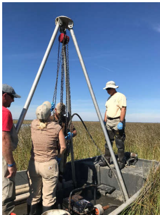
Greg supervises Jerome, Rob, Aaron, and Cooper (left) insert aluminum tube attached to vibracore. Alison hoists the tube using block and tackle mounted to tripod (right).
