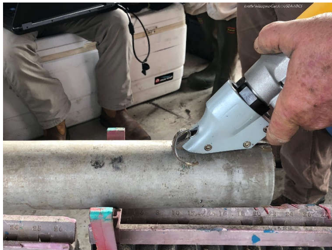
The aluminum tube is cut in half with electric shears.
