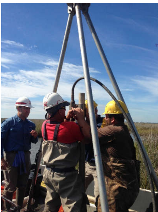
Greg supervises Jerome, Rob, Aaron, and Cooper (left) insert aluminum tube attached to vibracore. Alison hoists the tube using block and tackle mounted to tripod (right).
