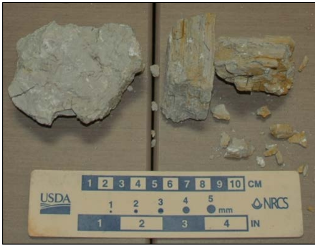
Within 10 minutes the mudstone showed signs of slaking. Chips of ~3mm in size were retained by the sieve. The large piece in the middle of the sieve continued to slake.
