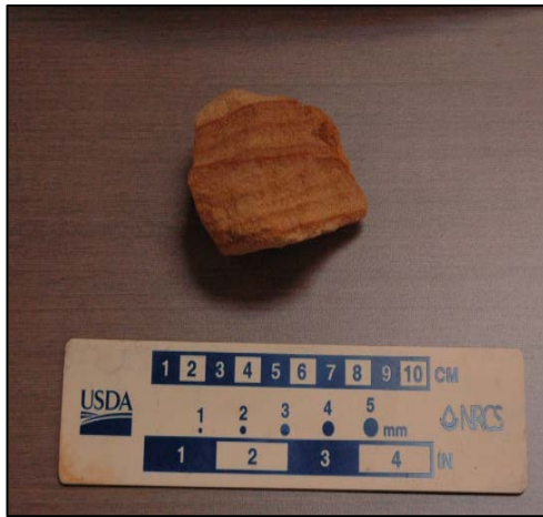
C material completely slaked and passed through a 2 mm sieve within 15 seconds.
