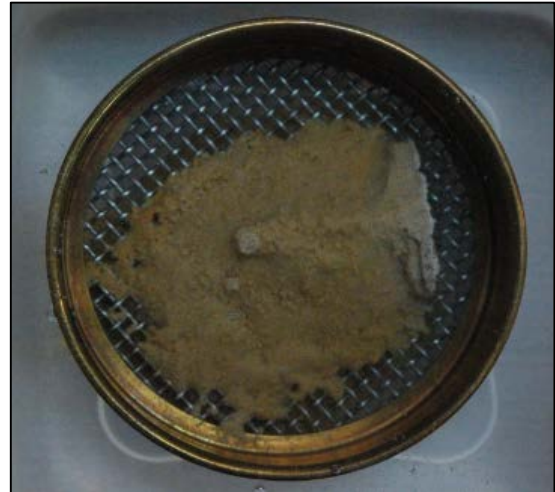
The sandstone readily slaked within 10 seconds. Interestingly, the upper part of the fragment (white colored material on the right side of the fragment) slaked more slowly probably due to some slight cementation by carbonates.
