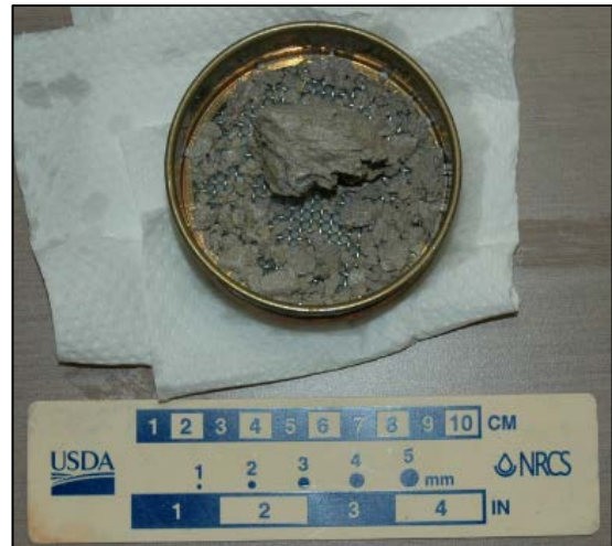
Within 10 minutes the mudstone showed signs of slaking. Chips of ~3mm in size were retained by the sieve. The large piece in the middle of the sieve continued to slake.
