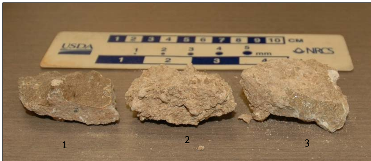
Samples from three different areas of the Petrocalcic Horizon. 1 (laminar cap) was indurated, 2 was non-cemented, and 3 was indurated.
