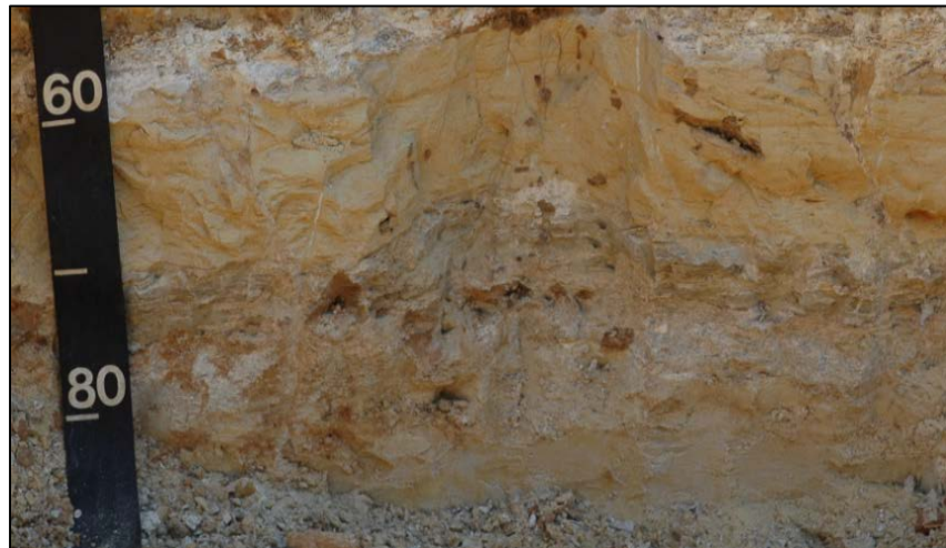
Non-cemented sandstone (commonly found in the Paluxy Formation)
